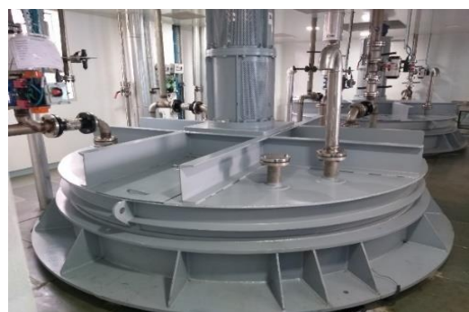
Blenders for the production of petroleum jellies at our Taloja Plant
