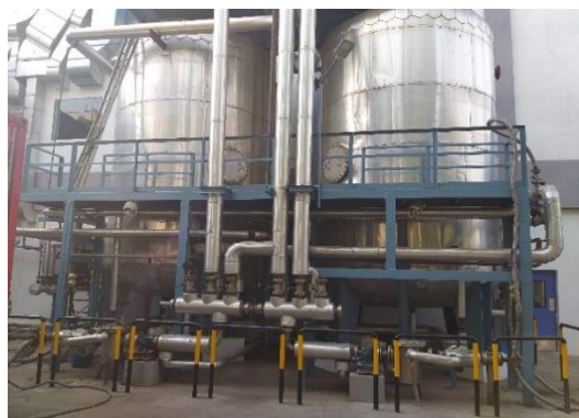
Blenders for the production of specialty oils at our Taloja Plant
