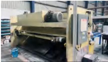
A large industrial shearing machine with a yellow body and a large metal blade, used for cutting metal sheets.                               |
