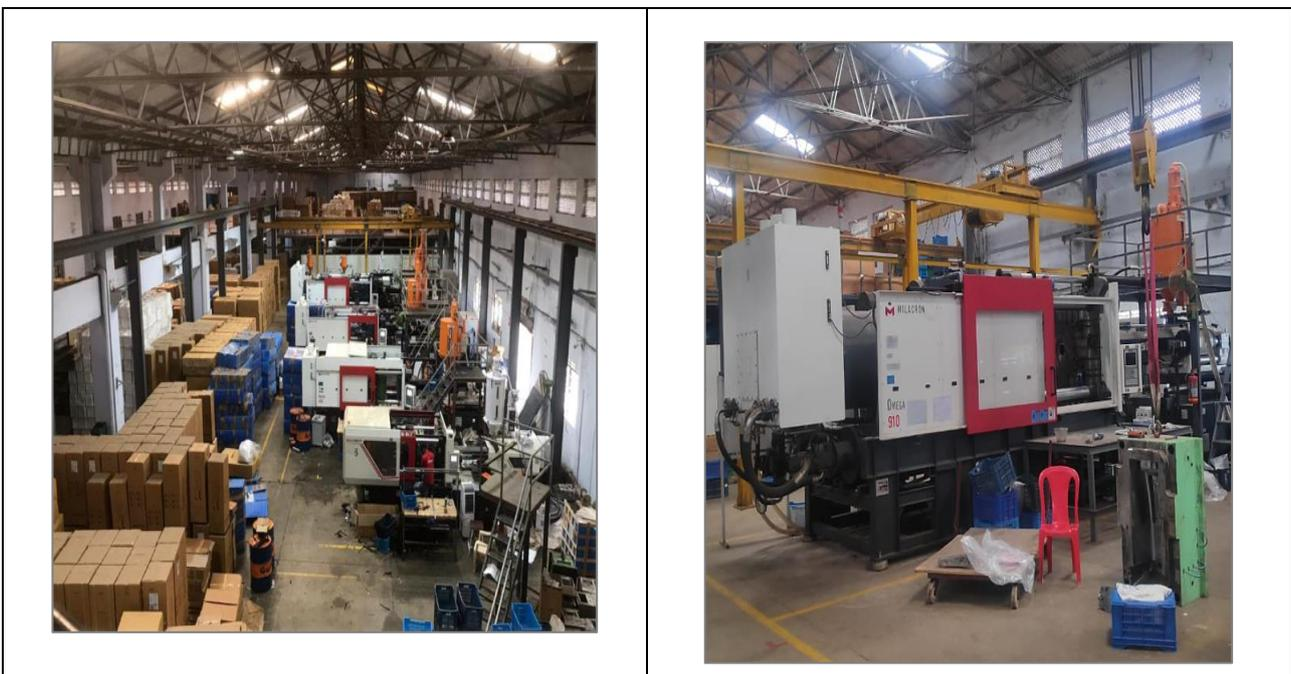
We have Moulding Unit Setup under same roof with 8 Moulding Machines- 3 of 100 Tons, 1 of 170 Tons, 1 of 280 Tons, 1 of 350 Tons, 1 of 450 Tons and 1 of 775 Tons.
