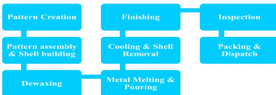
1. **Pattern Creation** - This initial step involves designing and creating a precise wax pattern that mirrors the final component. The pattern must be highly detailed to ensure accurate replication in the casting process.
