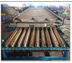
After shelling, the material is transferred to the vibratory sieve machine using an elevated feeder. This machine separates the cashew kernels (NW) from the shells due to the vibrations created by the sieve. The shells are then further segregated into uncut, semi-cut, and broken pieces using a roller.
