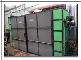
After drying the semi-processed kernels (NW), we need to add a small amount of moisture to enable easy removal of the husk. To achieve this, we place the kernels in moisture cabins before proceeding with the cashew husk removal process.
