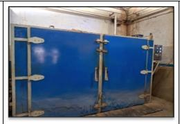
After obtaining the semiprocessed kernels (NW), we still need to remove the protective skin to get the final product. To do this, we dry the kernels for 8 hours, followed by an 8-hour cooling period. This process softens the husk layer, making it easier to peel, and also helps to dry out any excess oil, resulting in whiter kernels
