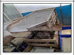
Once the husk is removed, the kernels are passed through this vibrator to separate the different pieces depending on the sizes.
