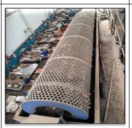
After the cooling of rcn, they are graded into basically 4 different sizes in descending order from D,C,B,A. The Sizing of the helps in proper and effective deshelling of the cashew nuts minimizing the quantity of broken kernels and increasing the quantity of whole cashew kernels.
