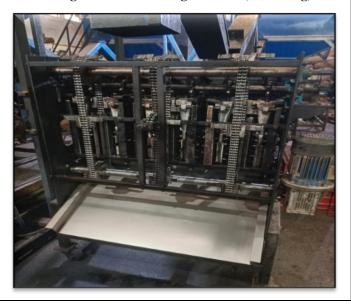
The cutting of raw cashew nuts (RCN) in our shelling machine is an operation essential for extracting kernels efficiently and minimizing waste. Our advanced shelling machines are configured to carefully crack open each nut, separating the shell from the kernel with precision. This process ensures maximum yield and maintains the integrity of the kernels, meeting our commitment to quality and efficiency in cashew nut processing.
