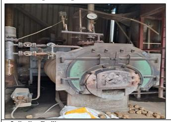
Steaming and boiling raw cashew nuts is a critical step in our processing, aimed at achieving optimal kernel extraction and quality. We control steam and boiling times to soften shells, facilitating kernel extraction while maintaining their nutritional content and natural flavor. Our precise steaming and boiling processes ensure that each batch meets our stringent quality standards, resulting in superior raw cashew nut products ready for further processing or distribution.
