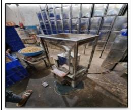
The cashew kernels are packed in tins using this machine, which also fills the tins with nitrogen gas. This process enhances the shelf life and quality of the cashew kernels.
