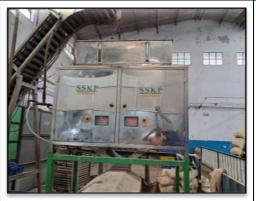
After giving the moisture to the nw, it is transferred to this machine for removal of husk, this machine uses the pneumatic technique to remove the husk from the cashew kernels before it could be processed further.
