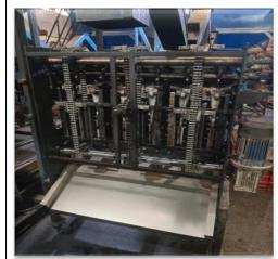
Shelling machines are used to deshell the raw cashew nuts (rcn) and obtain nw (semi-processed kernels) from the raw material. The raw material is segregated from the raw cashew grader and put in the machines on the basis of different size, each machine is caliberated for different sizes to obtain proper precision and 98% accuracy.
