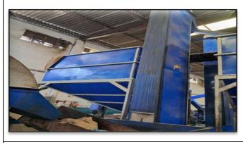
Our cooling facilities for raw cashew nuts (RCN) are designed to maintain optimal conditions after boiling. Post-boiling, RCN undergo controlled cooling to reduce moisture and oil content, which helps preserve freshness and quality. This controlled cooling process also facilitates the subsequent shelling step which prevents the spillage of oil during shelling, which may reduce the quality of the nuts.
