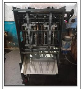
The raw cashew nuts (RCN) are de-shelled using shelling machines, producing semi-processed kernels (NW). The raw material is sorted by size using a raw cashew grader and then fed into the machines, which are calibrated to handle specific size ranges. Each machine is calibrated for different sizes to obtain proper precision and 98% accuracy.
