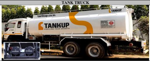
Tank trucks (top loading/ bottom loading) are customized as per customer requirements and a quality, durable, and efficient vehicles are designed for the safe transportation and handling of fuel. These are on-site assets and equipment to make the operation pilfer-proof, safe, and smooth with special safety features.
