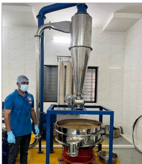
10-HP Masala Mill & Sifter Mesh Screen
